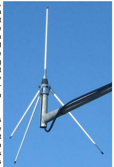
VHF ground plane antenna (2)
