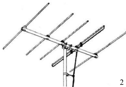
Drawing of Yagi–Uda VHF television antenna from 1954, used for analog channels 2–4, 54–72 MHz (U.S. channels)
