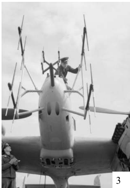
Quartet of two-dipole Yagi arrays (Hirschgeweih) of the German FuG 220 VHF-band radar on the nose of a late-World War II Bf 110 night fighter aircraft
