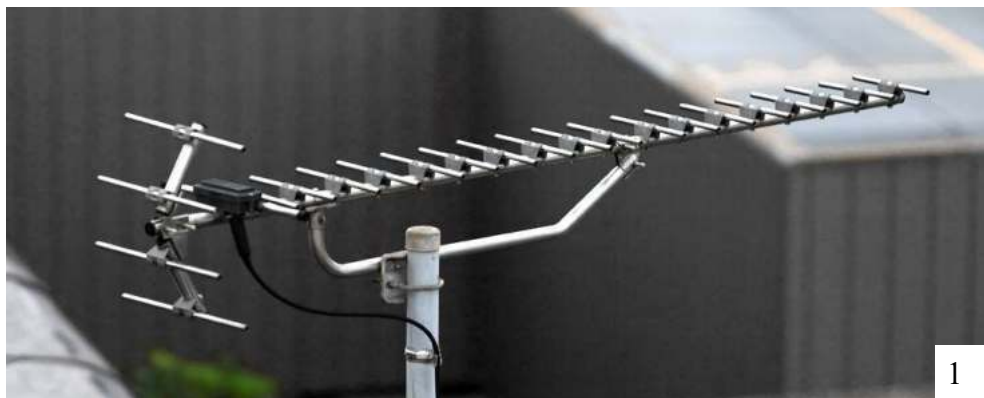
A modern high-gain UHF Yagi television antenna with 17 directors, and one reflector (made of four rods) shaped as a corner reflector.
