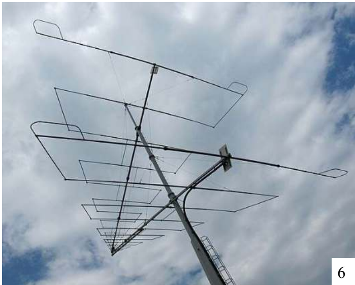
Wire log-periodic transmitting antenna at international shortwave broadcasting station, Moosbrunn, Austria. Covers 6.1–23 MHz.
