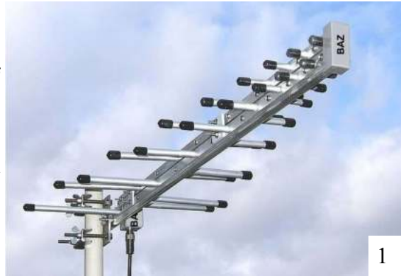
Log-periodic antenna, 400–4000 MHz
