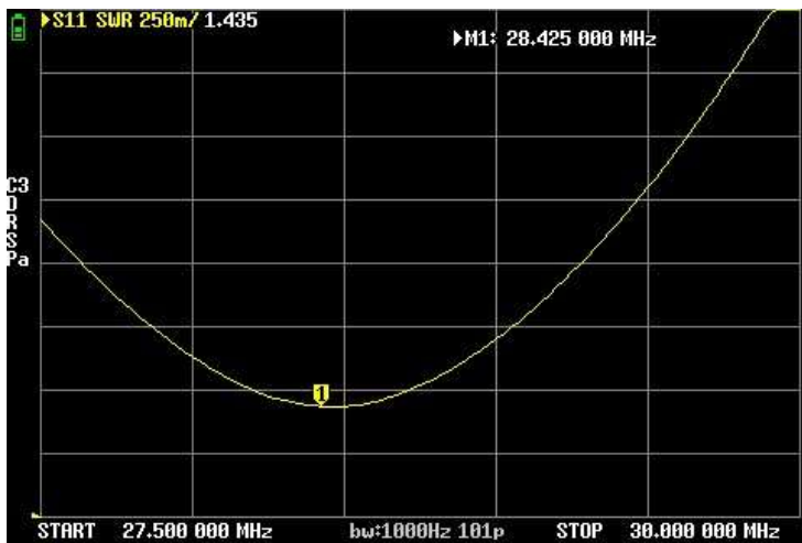
10m Band SWR 1.435 @ 28.425MHz
