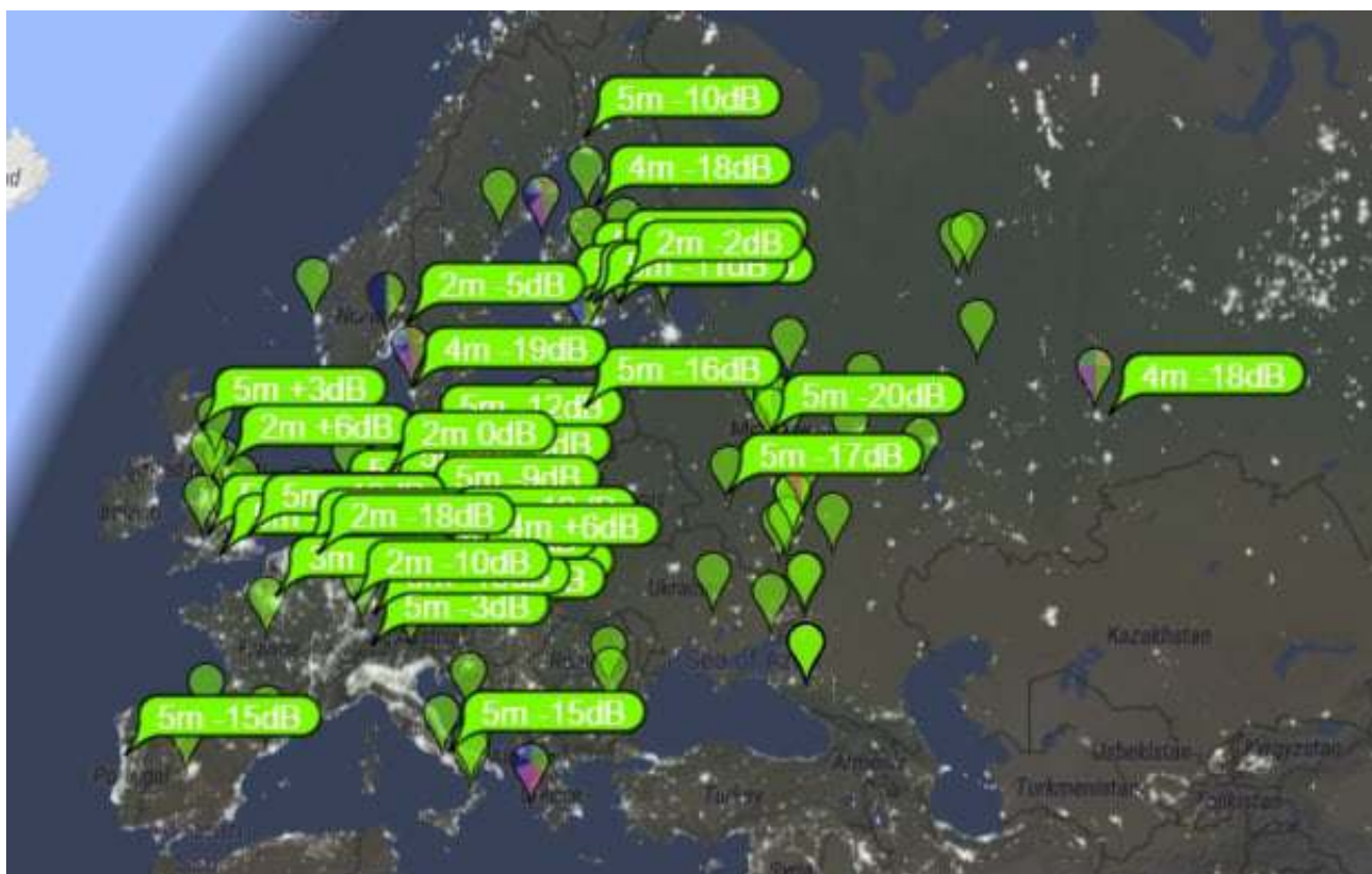
The Cobweb tuned to 160m band outperforming the 13m vertical
