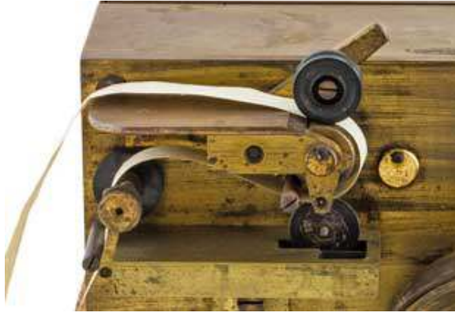
Paper feed on a Morse telegraph inker
