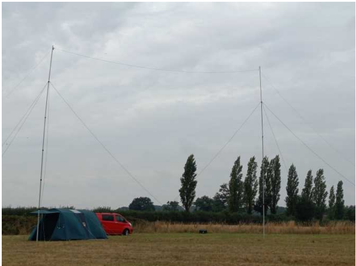
The OCF dipole, tent, Rogers van, and just about noticeable, the generator (centre picture).
