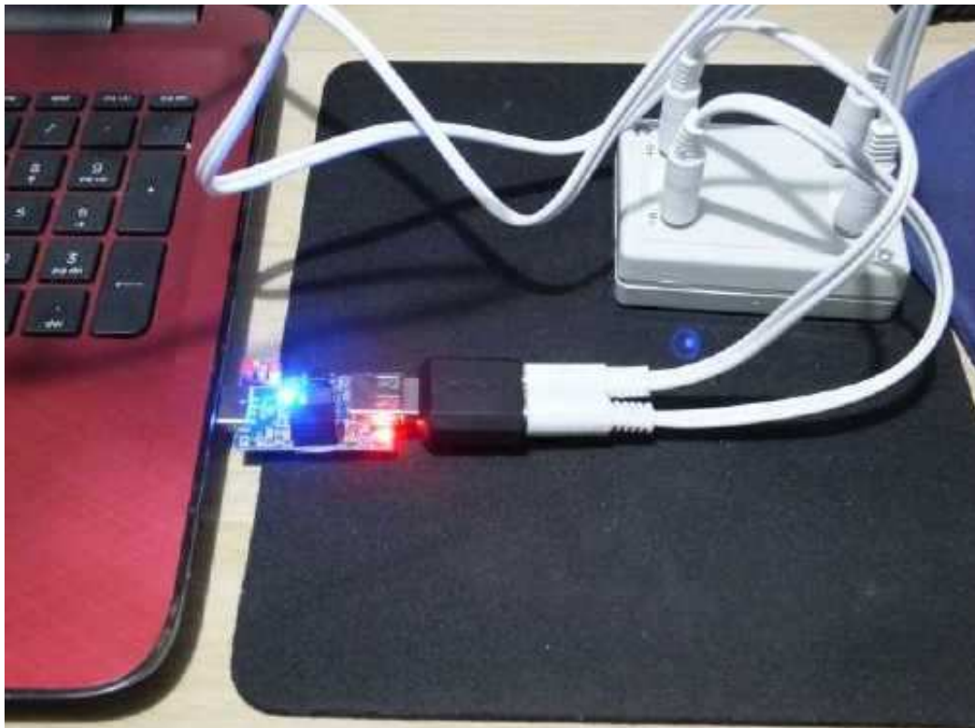
The sound is picked up from the 'Phones' socket, data transmitted via the 'Mic' socket.
