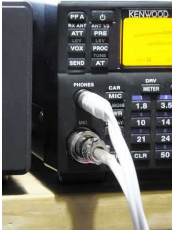
The sound is picked up from the 'Phones' socket, data transmitted via the 'Mic' socket.
