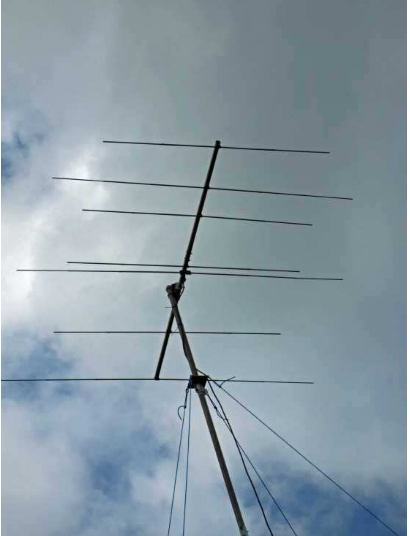
7. 4m/6m antenna was a PA5070-7-3 (Dual-band with 3 elements on 6m & 4 elements on 4m) from Antennas-Amplifiers of Serbia, courtesy of Roger (G3MEH).
