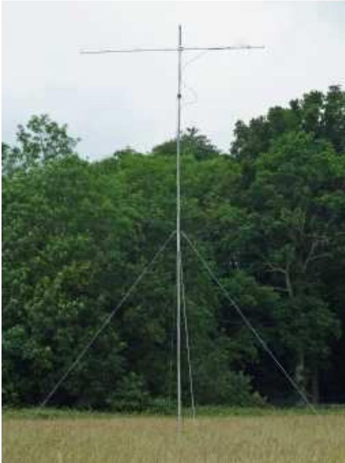
1. The first antenna to be erected, a 2m yagi, courtesy of G8FMC.
