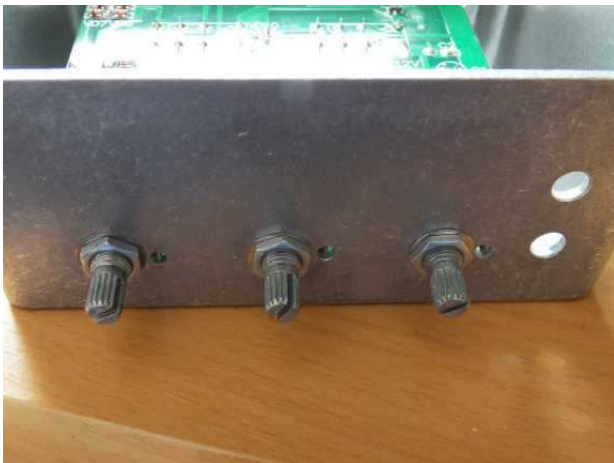
2. Controls and PCB installed.
