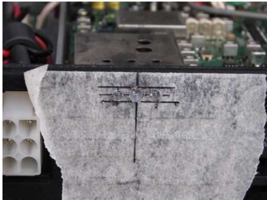
Marking up and drilling the back panel.
