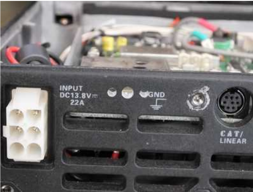
Now drilled and awaiting the SMA socket.
