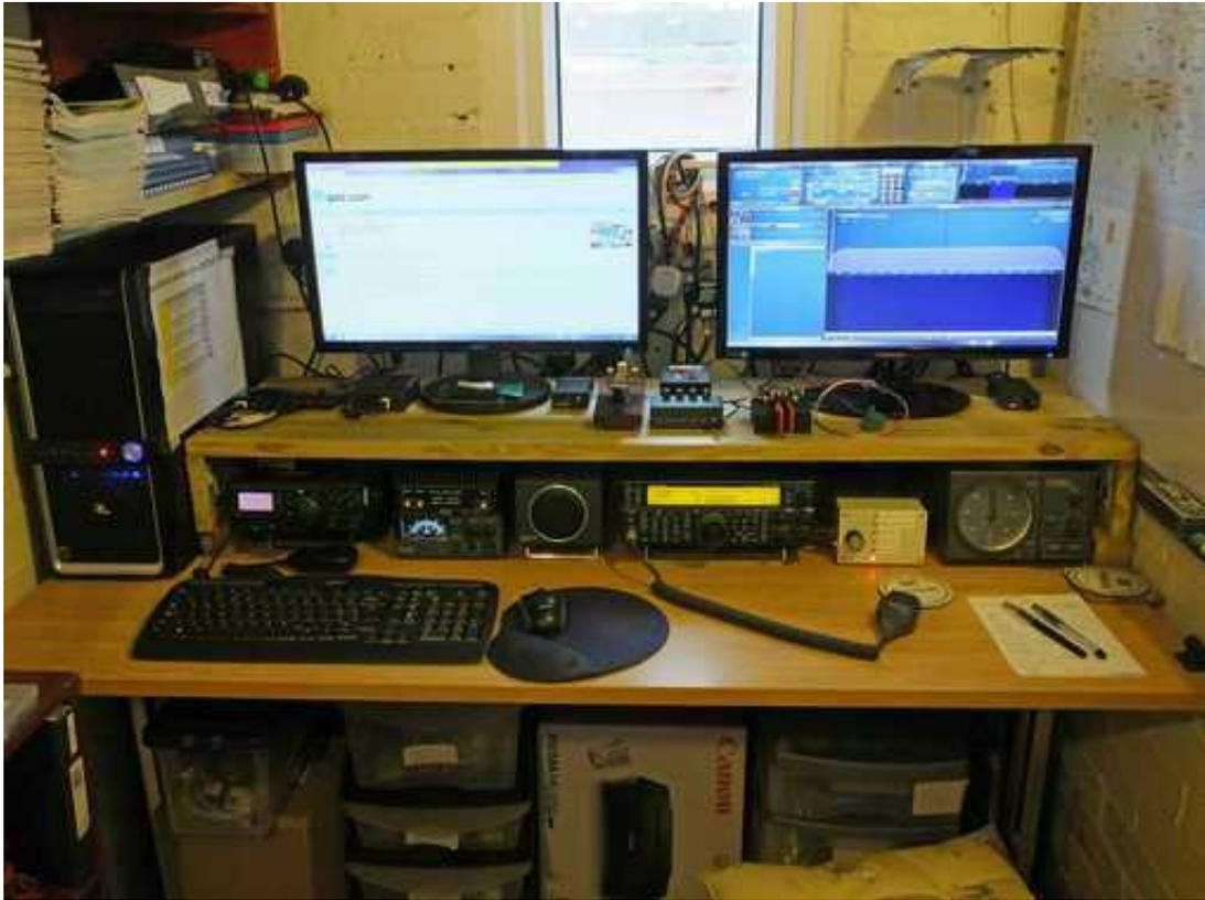
From left to right: Quad-core PC, TOP (left to right) - USB3 Hub, SDRPlay1a, DigiMaster CW Keying Interface, Kent 'straight' Morse Key, home-made CG3000 ATU Control box (back), headphone splitter (front), Begali paddle key, Digimaster GS232B Rotator PC Interface, BOTTOM - Yaesu FT-897D (Angie's), BNOS 432MHz Linear Amplifier (50W)(top), 32 amp PSU (bottom), SP23 speaker (Kenwood), Kenwood TS590SG, home-made antenna switch unit, Yaesu G-1000 DXC rotator controller.
